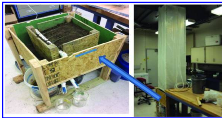
Figure 1. Photo of the soil slab reactor (left) and the rainfall simulation system (right) that was used for conducting the experiments.
